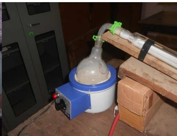
Fig.6 Early condensation on bend
